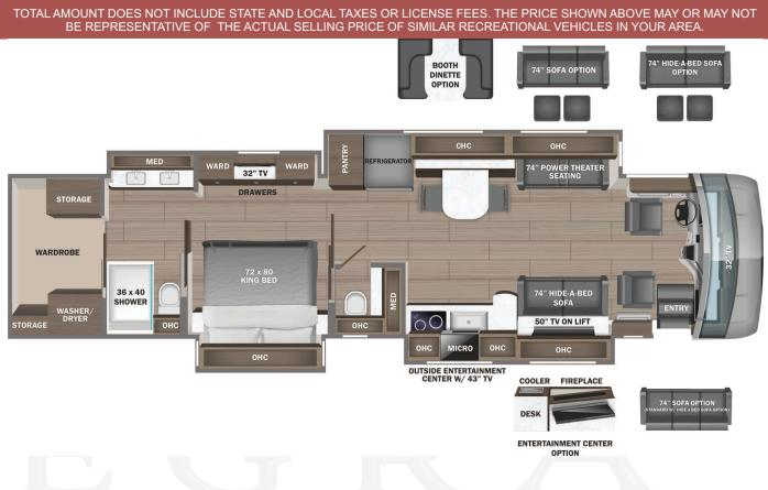
DIMENSIONS Exterior height:.....155.00" Exterior width:.....101.00"
